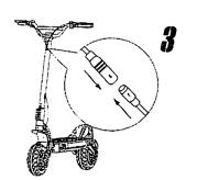
AFTER THE HANDLEBAR IS INSTALLED, FIND THE CONNECTORS CAREFULLY MATCH THEM BY COLOR. USING THE INDICATOR ARROWS ON BOTH SIDES CAREFULLY CONNECT THE TWO ENDS AND AVOID JAMMING ANY OF THE PINS.
