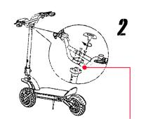
USING THE PROVIDED TOOLS, TIGHTEN THE 4 BOLTS ON THE HANDLEBAR. TIGHTEN EACH BOLT A FEW TURNS, THEN CONTINUE TIGHTENING UNTIL YOU REACH 75 INCH/POUNDS (8.5NM).
