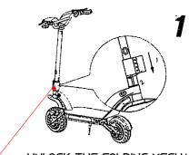
UNLOCK THE FOLDING MECHANISM AND SLIDE OVER THE FOLDING JOINT. MAKE SURE THE JOINT IS COMPLETELY COVERED BEFORE RE-TIGHTENING. WE RECOMMEND HAVING THE SCOOTER ON ITS KICKSTAND FOR INTIAL ASSEMBLY.
