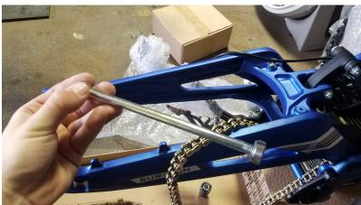
Step 10. Using your hand, slip the belt off the pulley side and onto the middle of the shaft. Do not slide belt to the outside, as it will become stuck.
