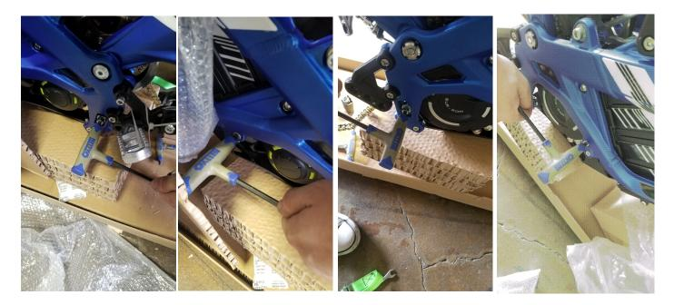
Step 5. Loosen Lock nut on half shaft bolt in preparation for removal.
