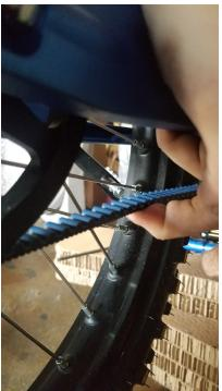
Step 35. Tighten down 17mm nut on rear axle and re check belt tension.
