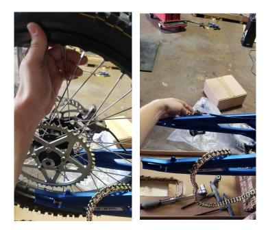
Step 4. Loosen motor mount bolts. There are 4 of them, 2 on each side of the frame, that hold the motor in.
