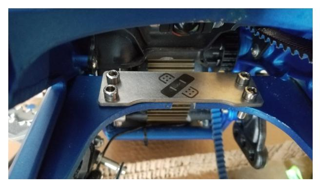
Step 30. Locate tensioning screws on the rear of the bike and adjust them in as far as they will go. This will make tensioning the belt possible, as it is shorter than the stock chain.
