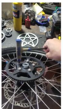
Step 18. Now that the half shaft is cool, install belt sprocket using stock 5mm bolts, tightening in a star pattern.
