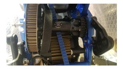
Step 23. Pry the left side belt onto the large pulley and rotate shaft while pushing belt onto pulley this will begin pull the shaft into place. At a certain point it will stick a little bit, but keep rotating and it will pop on.
