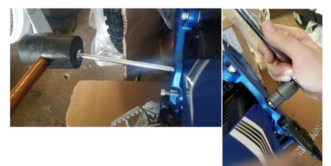
Step 27. Release motor mount bolt holding the motor up and tension the left side belt using the tensioner.
