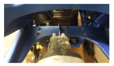
Step 21. Slip the belt through the cut in the pedal kit bracket and move to the side for now.
