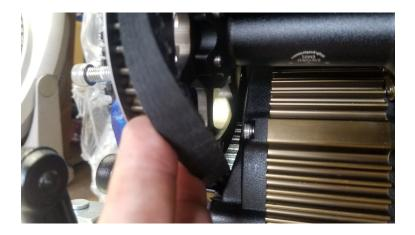
Step 11. Remove the Half Shaft. The shaft should pop out on most bikes, though blue Sur Rons seem to have a tighter fit than other colors. If you are unable to remove with a bit of wiggling and a firm tug, see set 11 a.
