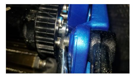
24 c. Use small flat head or Allen key to align bolt holes as much as possible, so that the shaft bolt will slide through.
