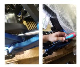
11c. Alternating left to right, and keeping the shaft as level as possible, gently tap the spacers until the shaft pops out.
