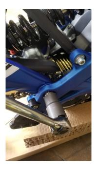
Step 6. Unbolt kickstand mount and set aside. This will get you the clearance needed to remove the shaft from the frame, otherwise the pulley will hit the kickstand and it will not come out.
