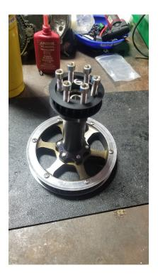
Step 19. Reinstall rubber grommet and shaft spacer. Be sure that the grommet is FLUSH with the new belt pulley, otherwise the spacer may slip out when installing shaft onto bike.
