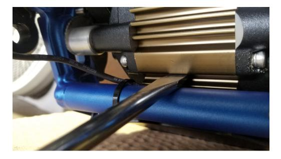
Step 9. Remove half shaft bolt and nut completely. DO NOT LOSE THIS PART!!!
