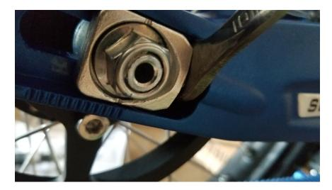
34a. Using the gates belt tension app (free on the google/iOS App Store) calibrate belt tension. (Tension should be between 80hz and 100 hz.
