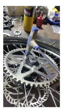
step 17. Install rear belt sprocket using stock 6mm bolts, tightening in a star pattern until the bolts snug up.
