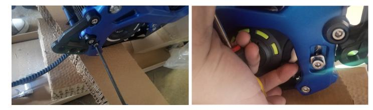
Step 28. Once tensioner is tight, tighten down all motor mounting bolts until they stop.
