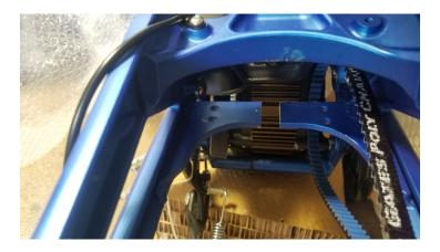
Step 22. Slip the belts onto the center of the half shaft and make sure nothing is pinching.
