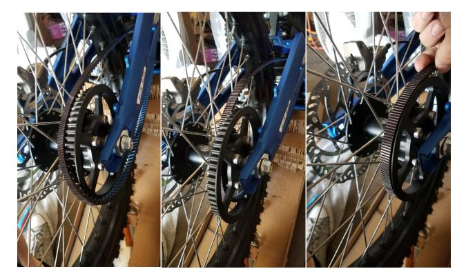
Step 34. Once the belt is seated on both pulleys, and the tension has been set on the motor, using the tensioner bolts and 10mm wrench, tension belt by turning bolts out evenly on both sides.
