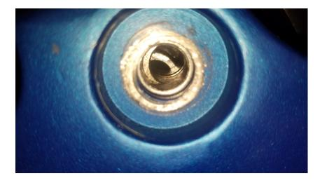
Step 25. Use a screwdriver or Allen key to align the holes for shaft bolt. Alignment must be near perfect or it will be difficult to slide the bolt through.
