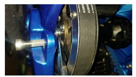
24 b. Using same method as removal, tap the spacers in evenly and slowly on both sides, being careful to keep shaft as straight as possible, until you are able to see the opening for the shaft bolt.
