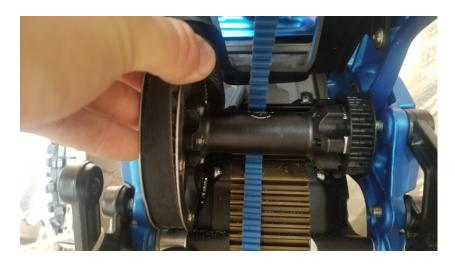
Step 24. Applying pressure to the spacers on either side of the half shaft, carefully slide it up into the frame and begin alignment of shaft. If you experience difficulty installing see step 24 a.
