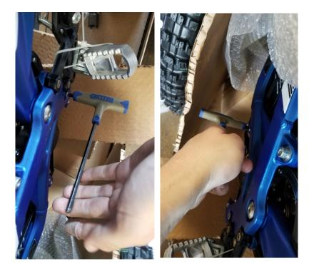
Step 29. Install luna band aid on the pedal mounting bracket that has been cut using supplied hardware and a 10mm wrench/4mm Allen key.
