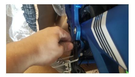
Step 33. Install the belt on to the wheel. Slide the belt over to the inside of the sprocket and push it onto the ridges, turning the wheel to feed the belt onto pulley.
