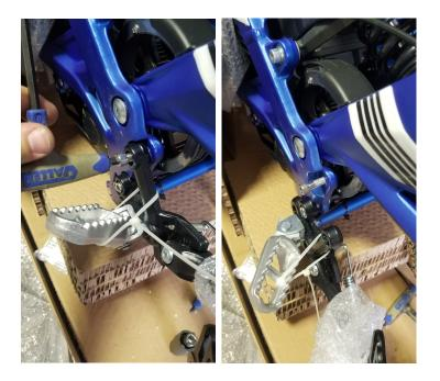
Step 7. Locate belt tensioner on the left side of the motor and disengage by pressing down. The slack will allow removal of shaft.
