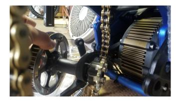
Step 12. Remove the chain by using either a flat head screw driver, or pliers, to release the clip on the missing link. The chain is easily removed once link has been released.
