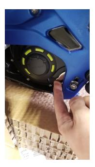
Step 8. Using pry bar or long screwdriver, lift motor and tighten down one of the rear motor mount bolt to hold in place. This will relieve tension on the belt allowing the half shaft to slip out much more easily.
