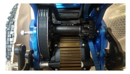
24 a. Line up spacers on either side of the shaft and work them into place, until shaft is in but not aligned. There i a bit of wiggle room in the spacers, and they can be slightly angled to fit into the frame. Once it can hang on its own you can begin working it into the frame.
