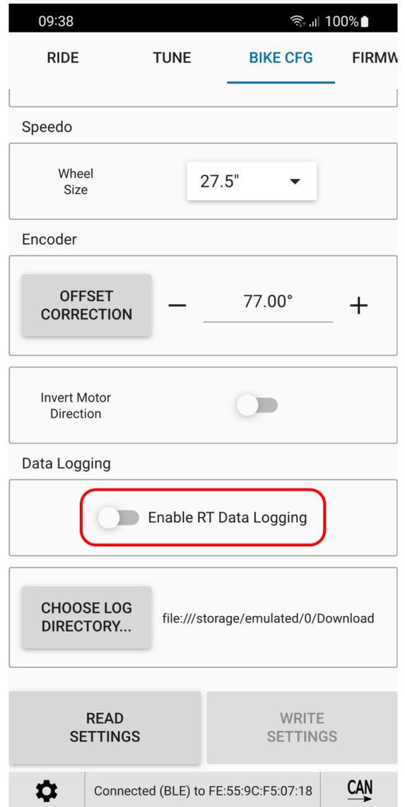
When datalogging is enabled, a .csv file will be created in the directory you configured. Each time logging is enabled, a new .csv will be created.
