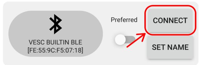
1. Turn ON the M600 from its display, open the VESC Tool App and start Scanning
