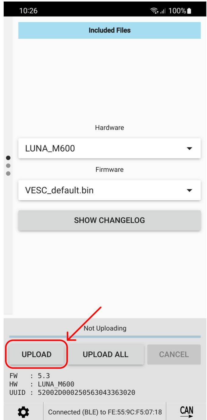
4. From the app, go to **FIRMWARE** tab and select the firmware according to your battery
