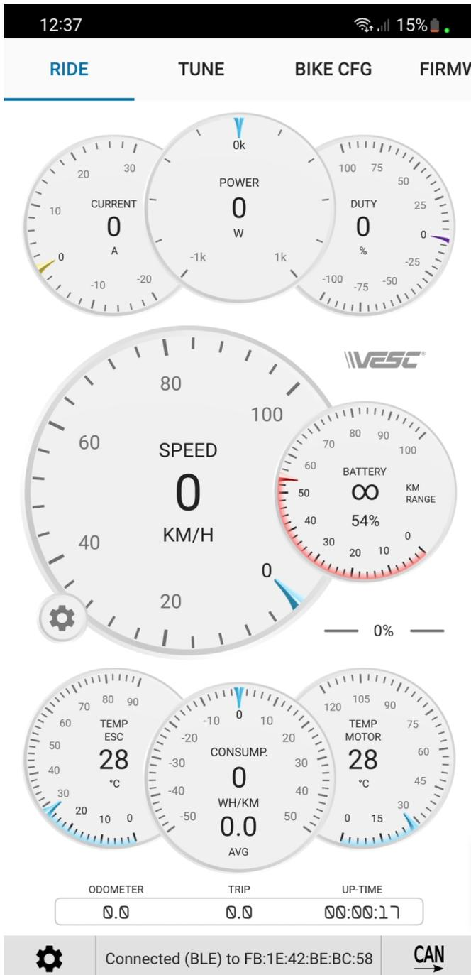
5. In the RIDE tab you can see live data coming from the controller. If you are pushing the bike hard, the motor temperature gauge is useful to avoid thermal throttling..
